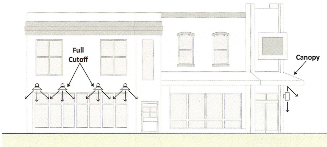
Figure 52: Exterior Light Shielding
