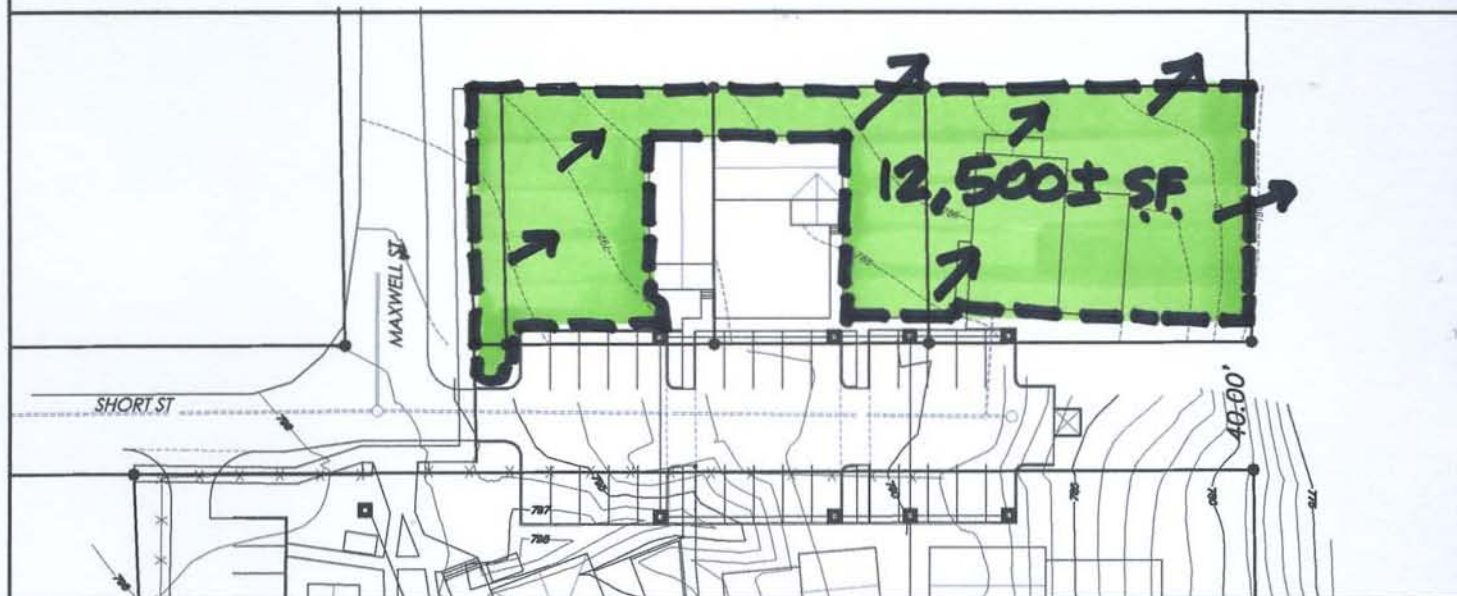
PROPOSED SURFACE DRAINAGE AREA-1
