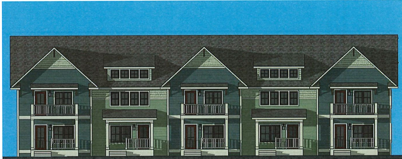
FRONT ELEVATION SCALE: 3/32" = 1'-0"
