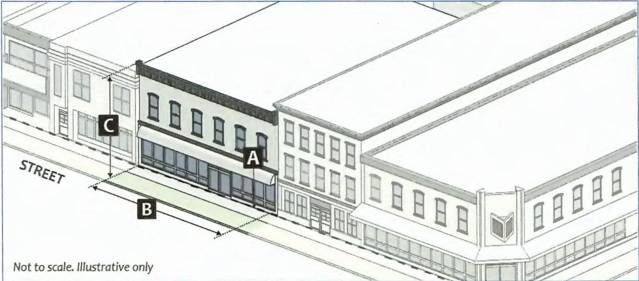
Figure 28: MD-CS Downtown Character Overlay Dimensional Standards
