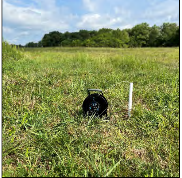
Photo 2: Piezometer installed at B-3; View to the north
