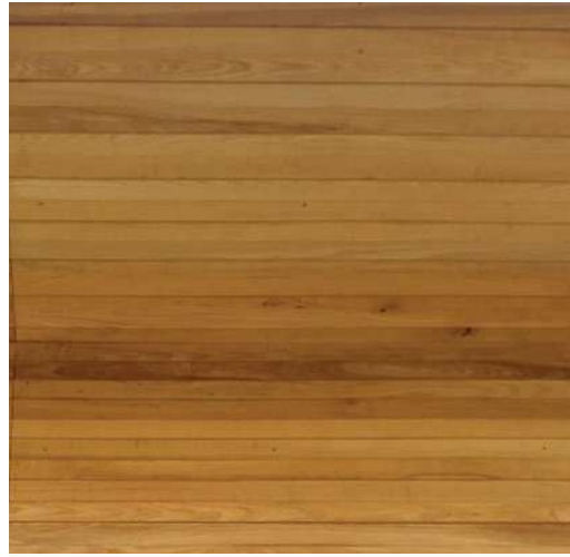
ASH - SOFFIT MATERIAL
