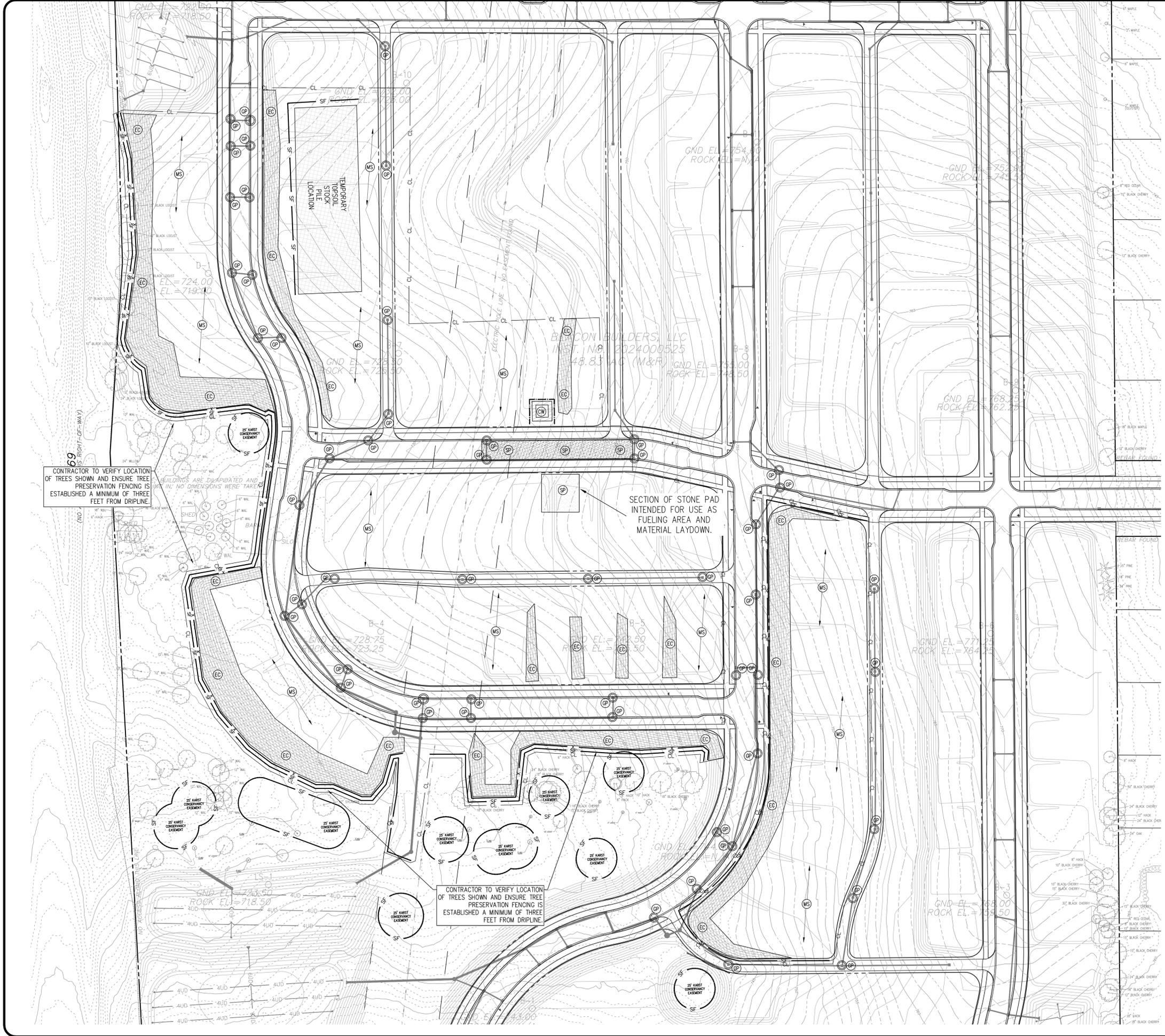
CONTRACTOR TO VERIFY LOCATION OF TREES SHOWN AND ENSURE TREE PRESERVATION FENCING IS ESTABLISHED A MINIMUM OF THREE FEET FROM DRIFLINE.
