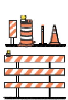
1. Stripes on barricade rails slope downward at an angle of 45 degrees toward the direction traffic is to pass.
