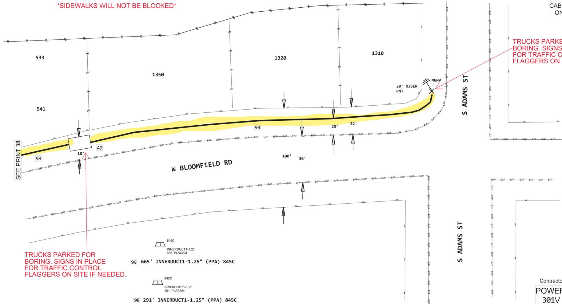
TRUCKS PARKED FOR BORING. SIGNS IN PLACE FOR TRAFFIC CONTROL. FLAGGERS ON SITE IF NEEDED.
