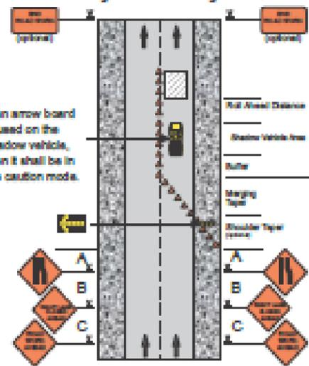
If an arrow board is used on the shadow vehicle, then it shall be in the caution mode.
