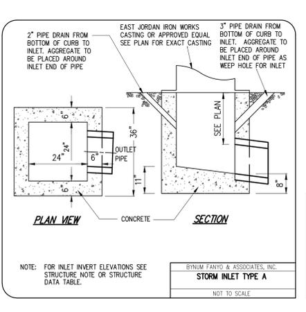
**NOTE: ALL DOUBLE OR TRIPLE INLETS TO BE INTERCONNECTED BY DUAL WALL TYPE 'S' HDPE PIPE WITH A LENGTH OF ONE FOOT AND DIAMETER EQUIVALENT TO THAT OF THE ASSOCIATED OUTLET PIPE.**
