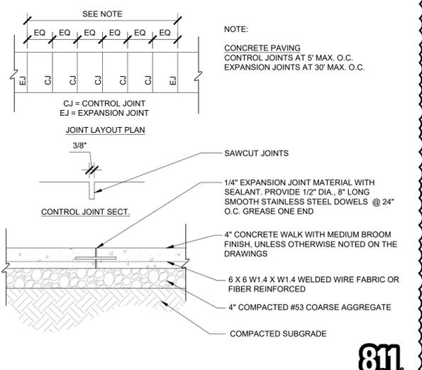
**1 STANDARD CONCRETE PAVEMENT & JOINT**
