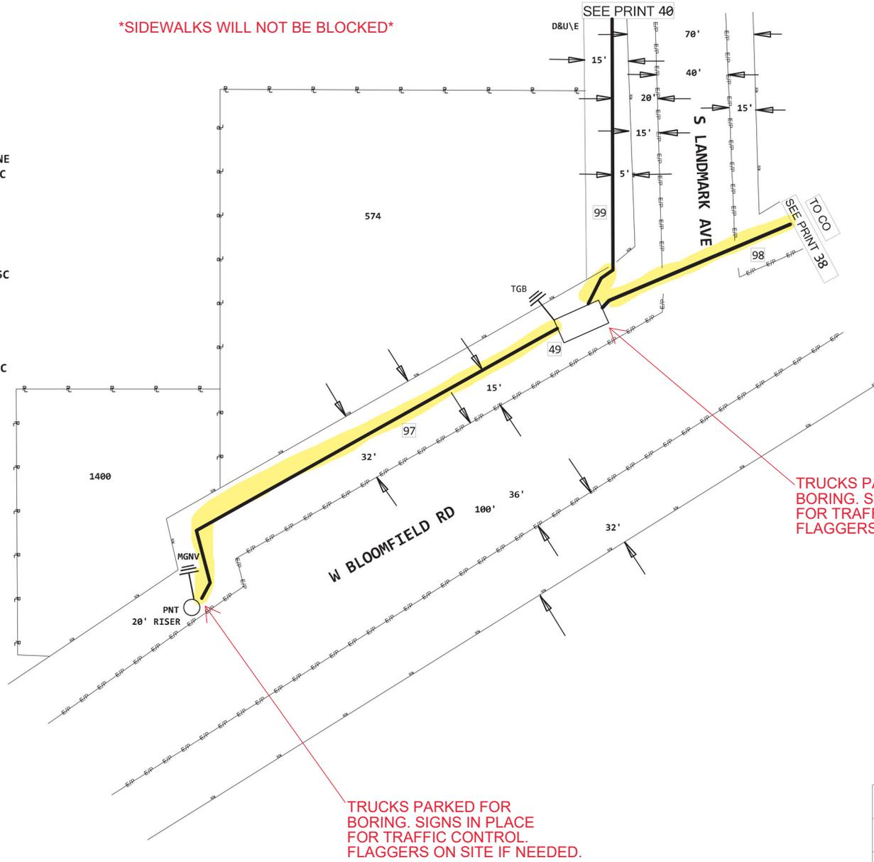
TRUCKS PARKED FOR BORING. SIGNS IN PLACE FOR TRAFFIC CONTROL. FLAGGERS ON SITE IF NEEDED.
