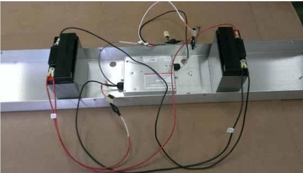
Figure 6. Batteries Wired in Parallel
