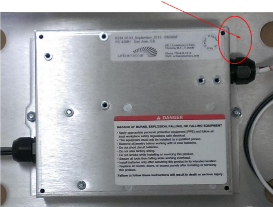
The Switch is now mounted on the inside wall of the chassis of the power module unit so that it can be enabled by swiping a magnet on the outside wall of the unit as shown in the following photos. The TEST location will be clearly labelled so that maintenance staff can quickly check the status of the unit without opening or removing any of the system covers.
