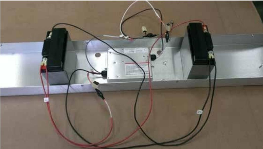
Figure 6. Batteries Wired in Parallel
