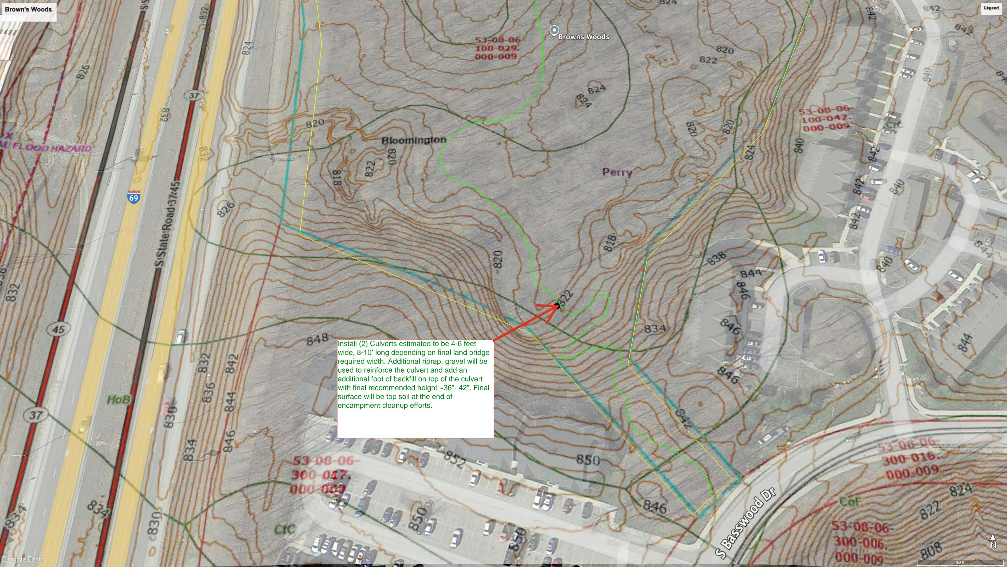
Install (2) Culverts estimated to be 4-6 feet wide, 8-10' long depending on final land bridge required width. Additional riprap, gravel will be used to reinforce the culvert and add an additional foot of backfill on top of the culvert with final recommended height ~36"- 42". Final surface will be top soil at the end of encampment cleanup efforts.
