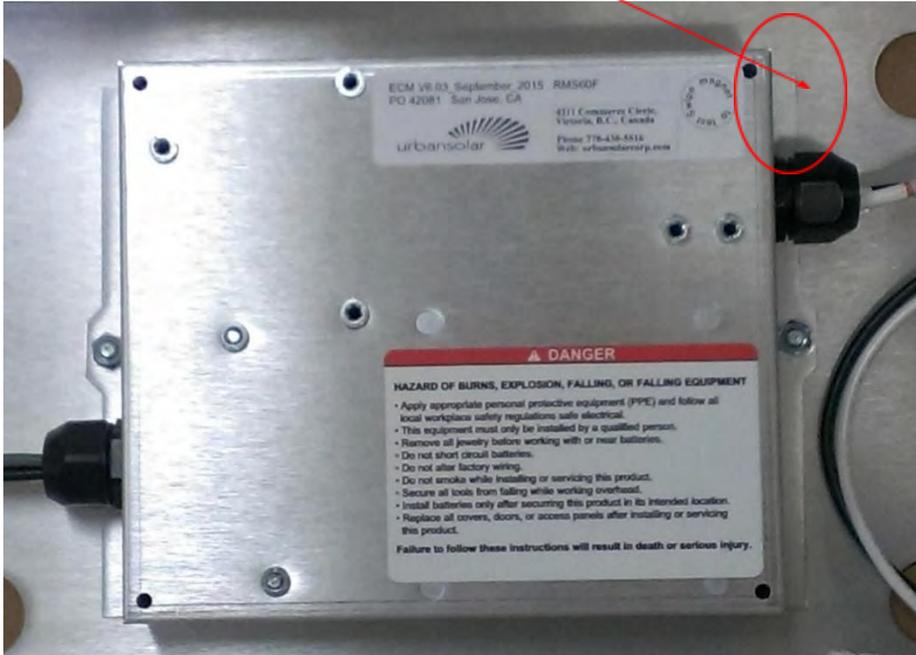
The Switch is now mounted on the inside wall of the chassis of the power module unit so that it can be enabled by swiping a magnet on the outside wall of the unit as shown in the following photos. The TEST location will be clearly labelled so that maintenance staff can quickly check the status of the unit without opening or removing any of the system covers.
