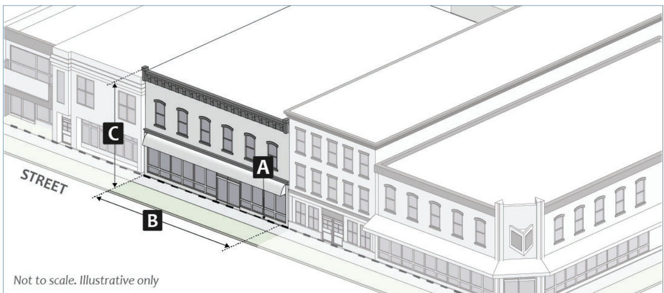
Figure 28: MD-CS Downtown Character Overlay Dimensional Standards
