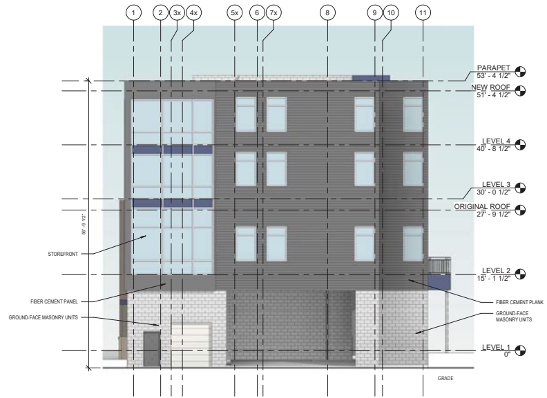
SOUTH ELEVATION 1/8" = 1'-0" NORTH
