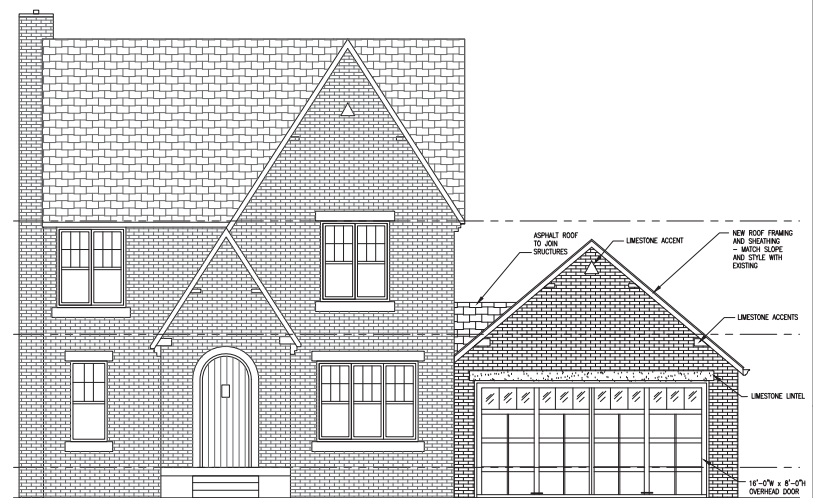
2 PROPOSED SOUTH ELEVATION 1/4" = 1'-0"
