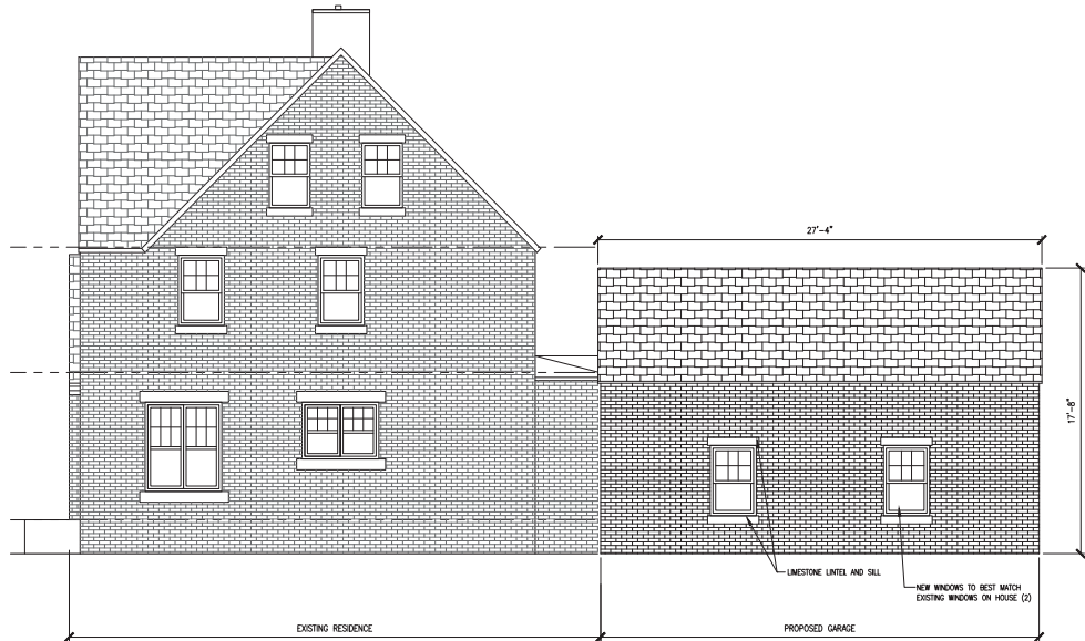
1 PROPOSED EAST ELEVATION 1/4" = 1'-0"
