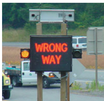
When the sensors determine a vehicle is traveling the wrong way, the message sign illuminates a red "Wrong Way" message (right).
