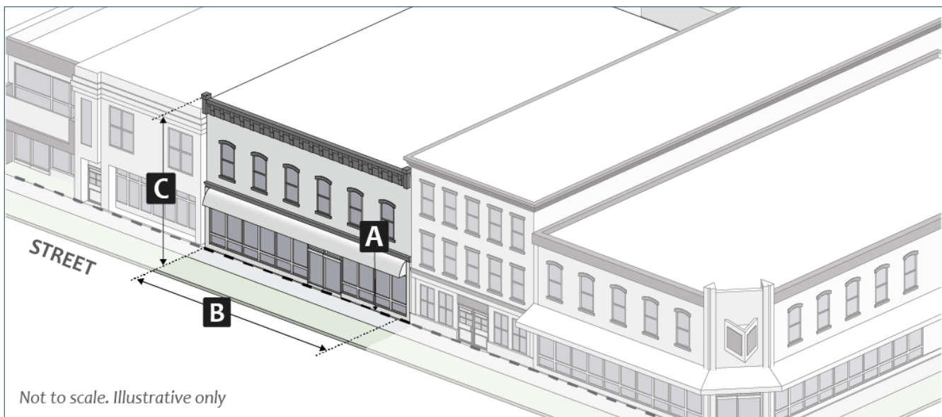
Figure 28: MD-CS Downtown Character Overlay Dimensional Standards
