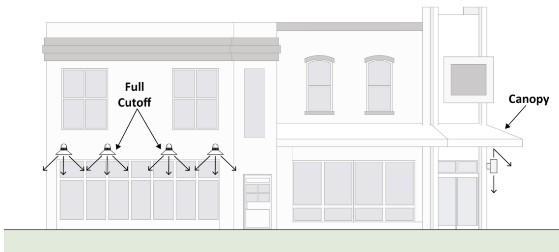
Figure 52: Exterior Light Shielding
