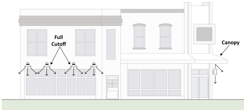
Figure 52: Exterior Light Shielding
