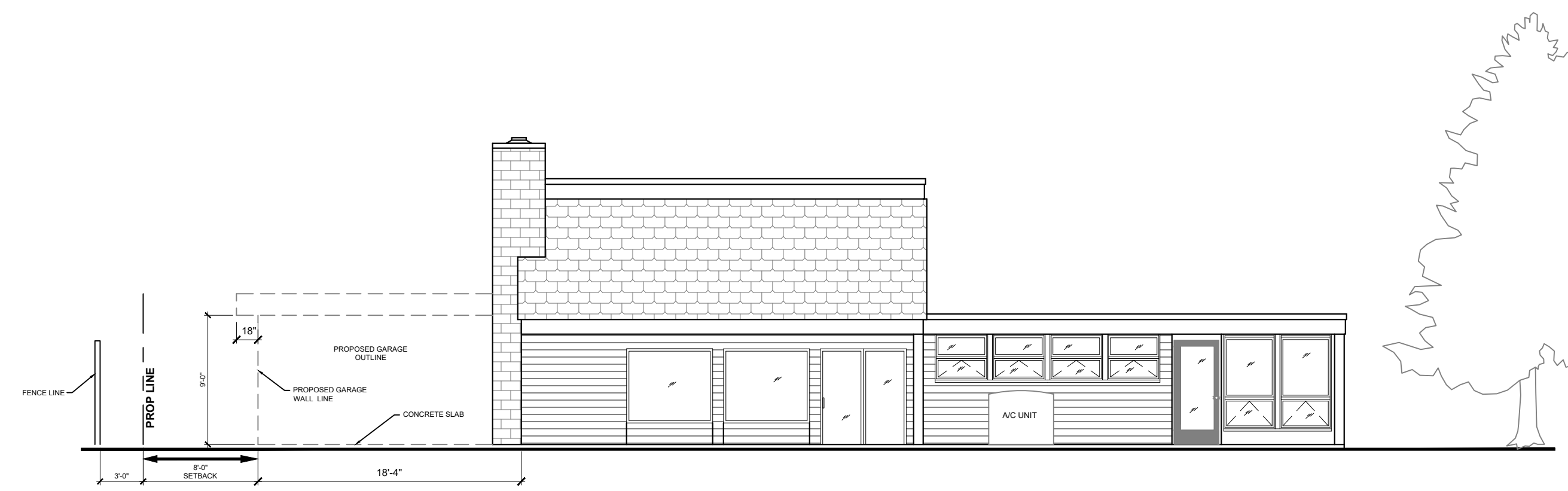
NORTH ELEVATION - EXISTING WITH PROPOSED GARAGE OUTLINE
