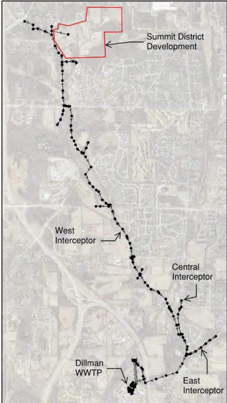
Figure 1-1: Dillman WWTP West Interceptor SWMM Hydraulic Model
