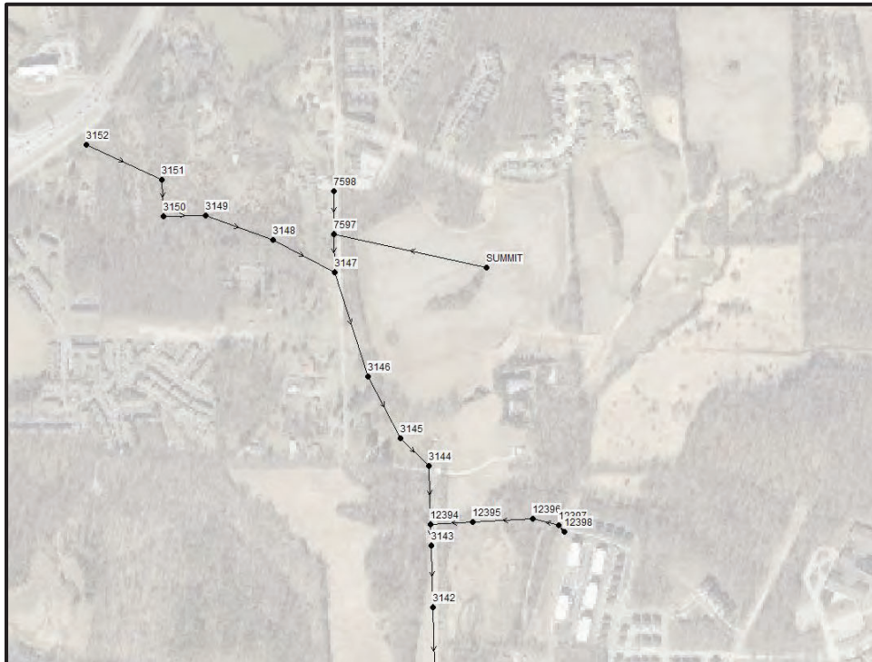
Figure 3-1: Summit District Connection to Existing Collection System
