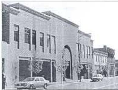
Locate the front building wall at the sidewalk line when feasible. (Bloomington, IN)
