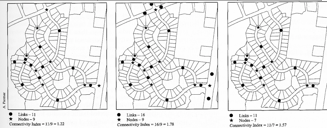
Figures 3.3A, 3.3B, and 3.3C. (Left) Cary rules: Include nodes with arterials but no external links. (Center) Orlando rules: Include nodes with arterials and one link beyond the last node. (Right) San Antonio, Concord, and Hillsborough rules: Do not include nodes on arterials.
