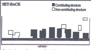
Set-back zone for new residential structures should be determined by the set-back ranges of contributing houses on that block, as shown by the grey band in this drawing.
