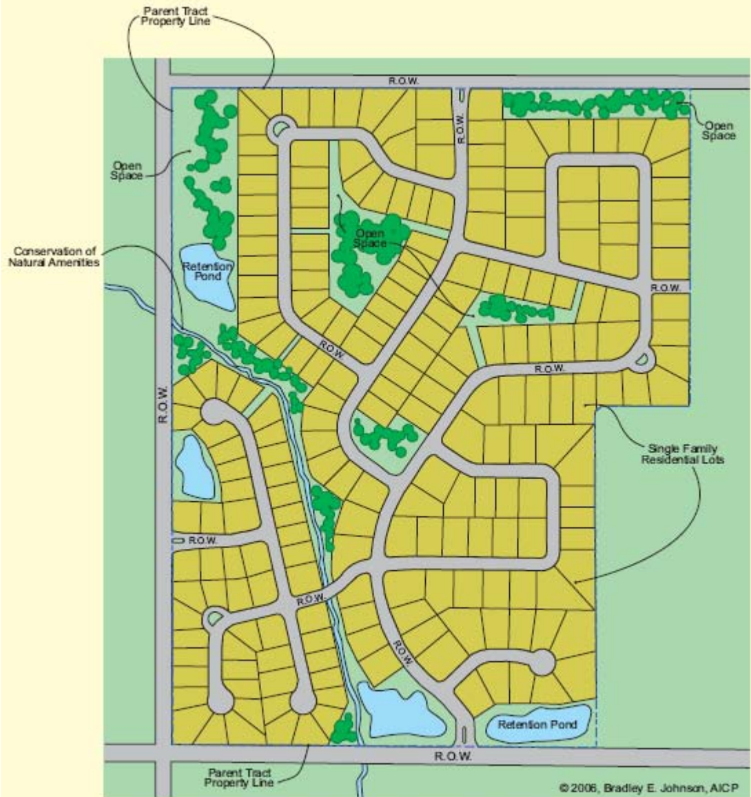
The diagram above is intended to illustrate the concepts outlined in this Chapter. The design of new subdivisions must follow the regulations of the Unified Development Ordinance, but need not match this illustration.
