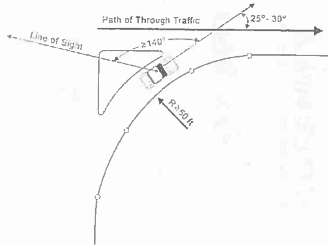
a. Traditional design: Requires driver to rotate head and body through a large angle to observe approaching vehicles.
