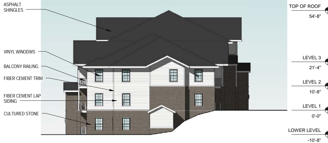
2 BUILDING 2 - SOUTH ELEVATION A2.5 1/16" = 1'-0"
