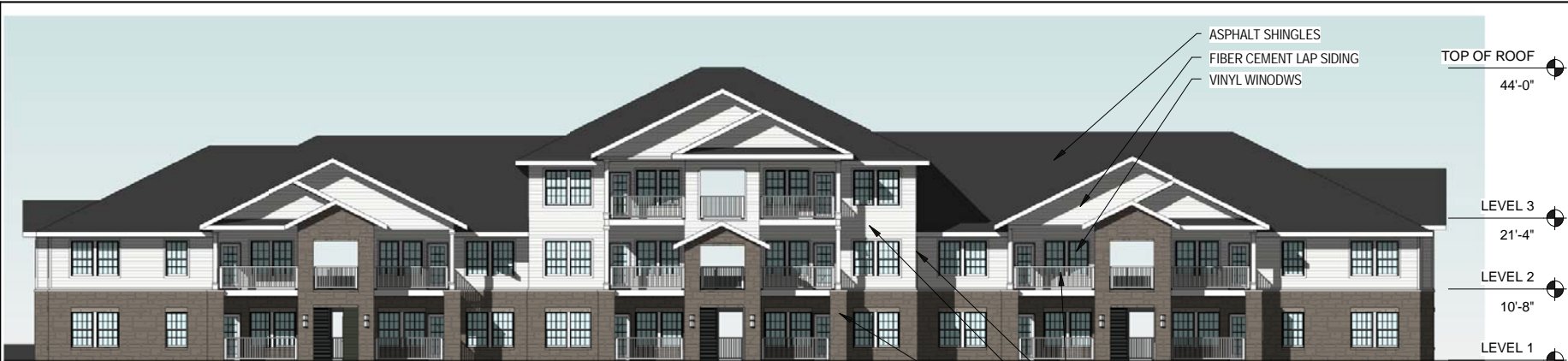
1 BUILDING 2 - EAST ELEVATION A2.4 1/16" = 1'-0"
