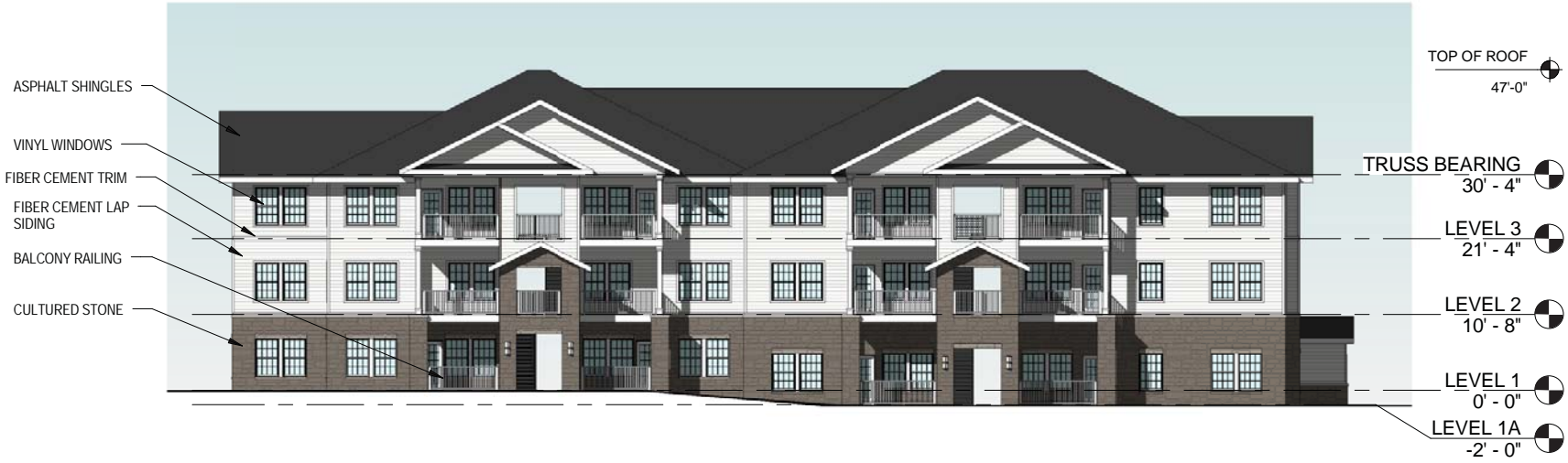
2 BUILDING 1 - EAST ELEVATION A1.4 1/16" = 1'-0"
