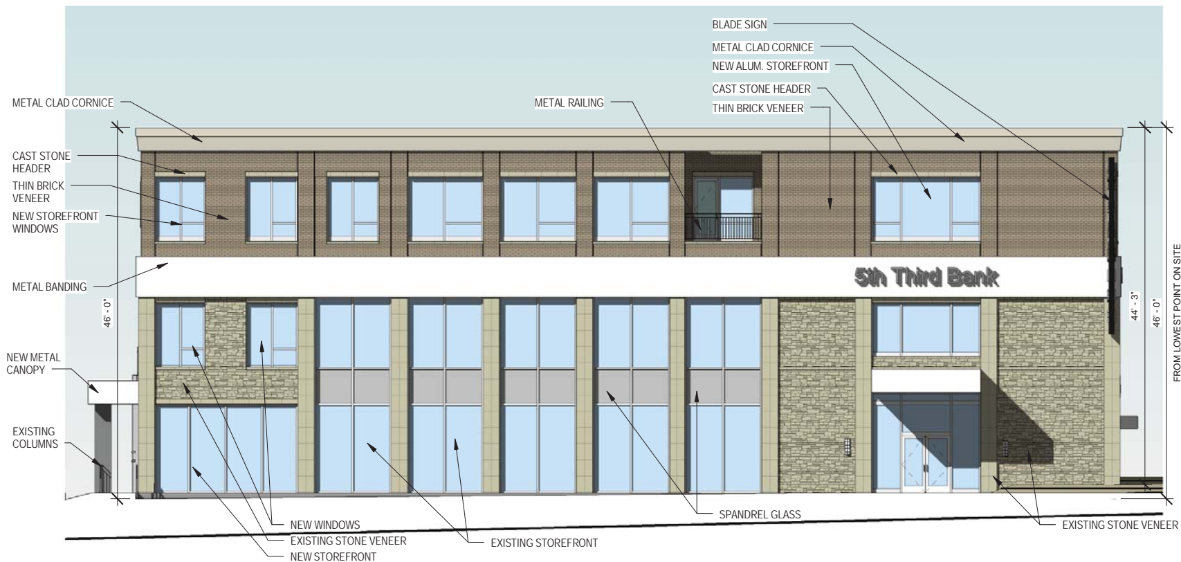
1 BLDG 2 - EAST ELEVATION - WASHINGTON ST. A10 3/32" = 1'-0"
