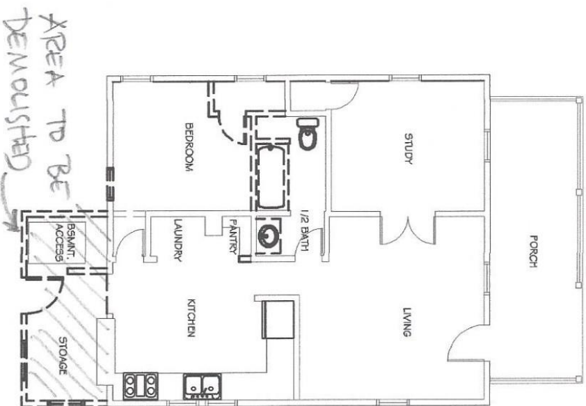
A DEMOLITION FLOOR PLAN
