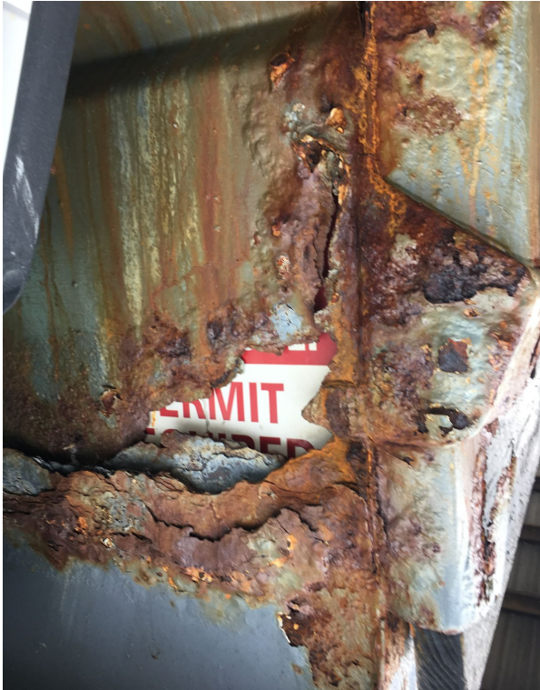
Close up of rusty truck bed (patched with old street sign)
