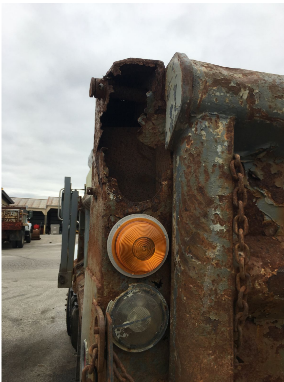
Close up of rusty truck bed (patched with old street sign)
