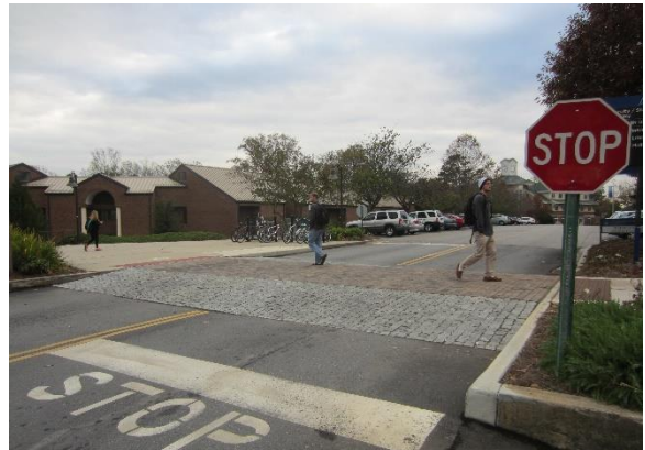
Raised crosswalk example
