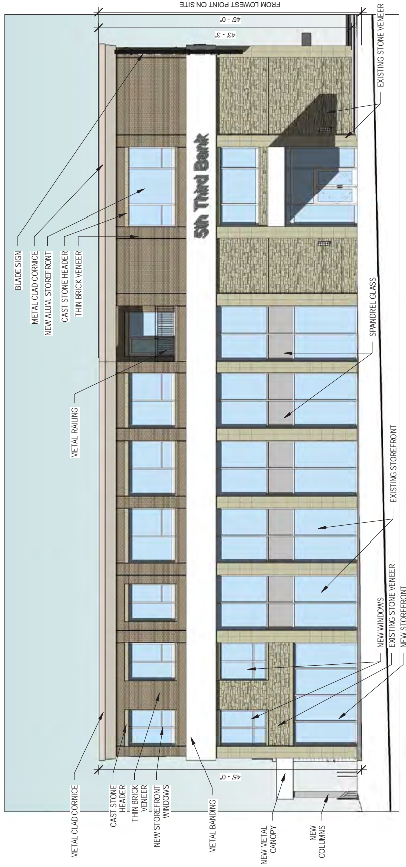
1 BLDG 2 - EAST ELEVATION - WASHINGTON ST. A10 3/32" = 1'-0"
