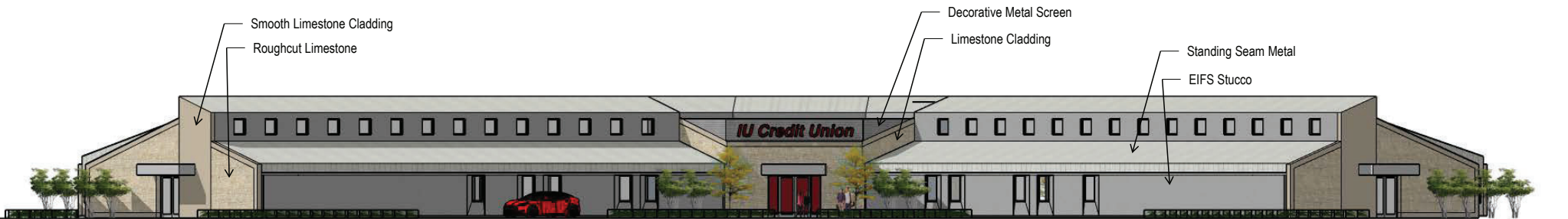
South Elevation – Main Entry facing Hagan
