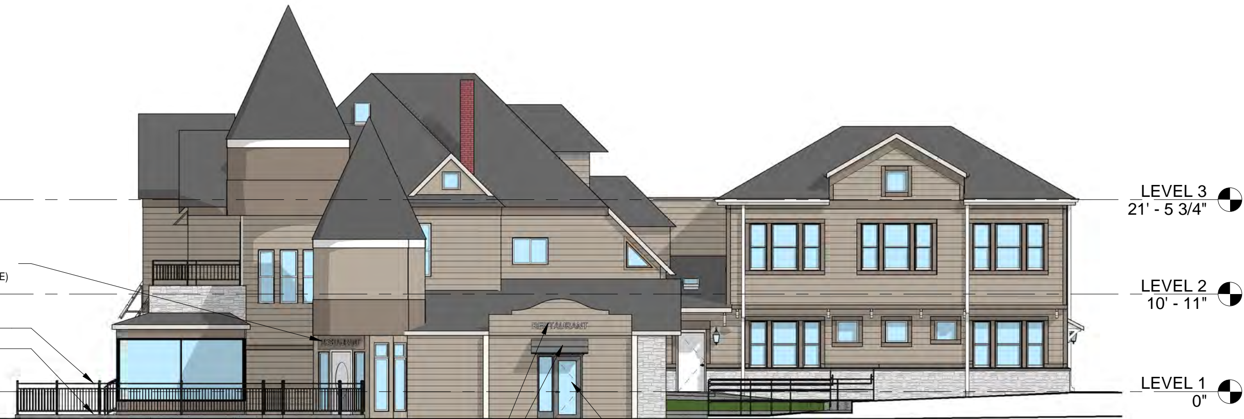
2 EAST ELEVATION - 1 2 3/32" = 1'-0" NEW PAINTED METAL LETTERS ON STAND OFFS W/ BACKLIGHTING (TENANT SIGNAGE) NEW DARK FABRIC AWNING NEW ADA ACCESSIBLE TENANT ENTRY DOOR
