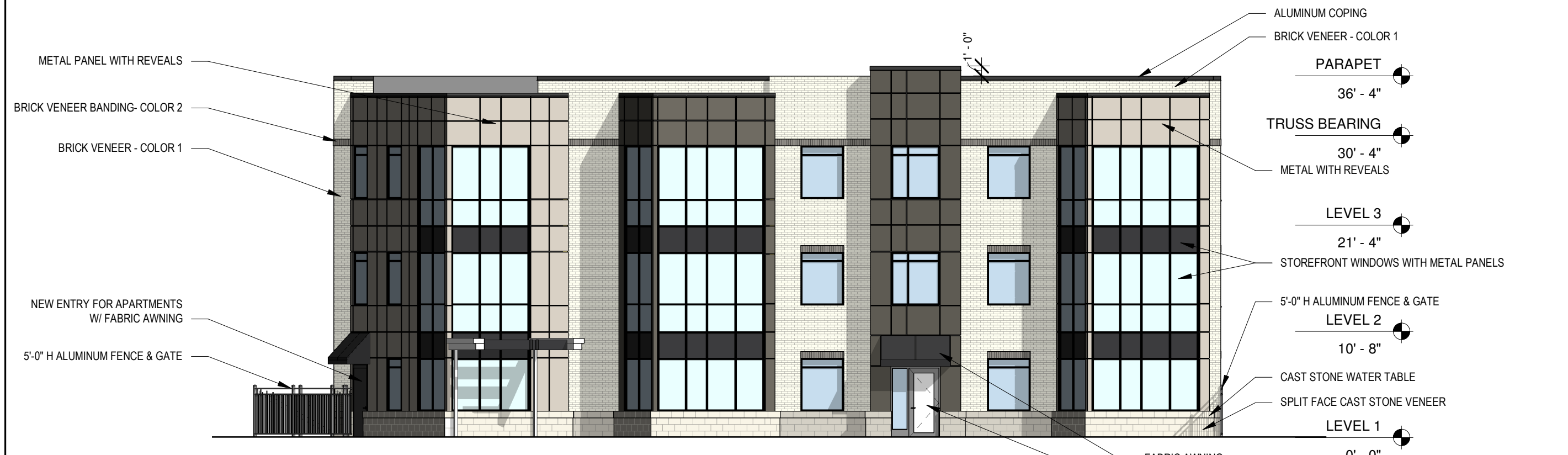
1 SOUTH ELEVATION - COURTYARD A8 3/32" = 1'-0"
