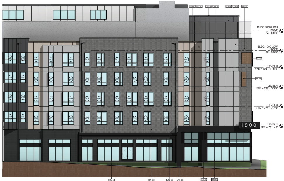
3 BLDG 1000 - WEST ELEVATION PART C 1/8" = 1'-0"
