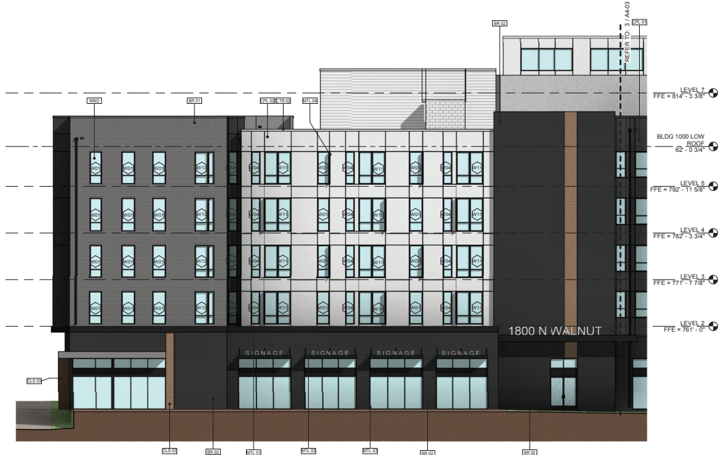
1 BLDG 1000 - WEST ELEVATION PART B 1/8" = 1'-0"
