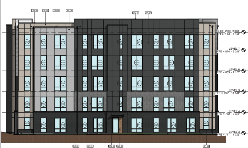
2 BLDG 2000 - EAST ELEVATION PART E 1/8" = 1'-0"
