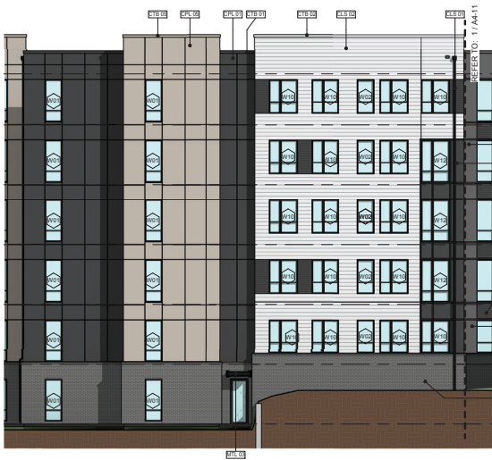
5 BLDG 2000 - SOUTH ELEVATION PART D2 1/8" = 1'-0"
