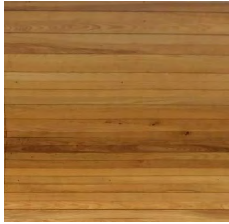
ASH - SOFFIT MATERIAL
