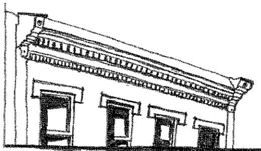
Full cornice restoration based on sufficient evidence.
