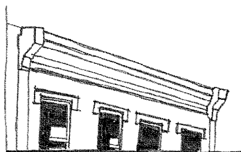
Simplified cornice constructed where evidence is insufficient
