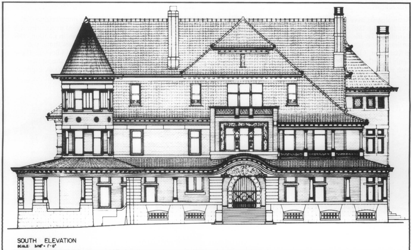
Figure 1. Clay tiles used as roof covering and as vertical cladding on the third story and gable ends are important in defining the historic character of the Alfred W. McCune Mansion in Salt Lake City. Designed by the architect S.C. Dallas, and completed in 1901, this brick and brownstone structure is a tiled variation of the Shingle style. Drawing: Clay Fraser, HABS Collection.
