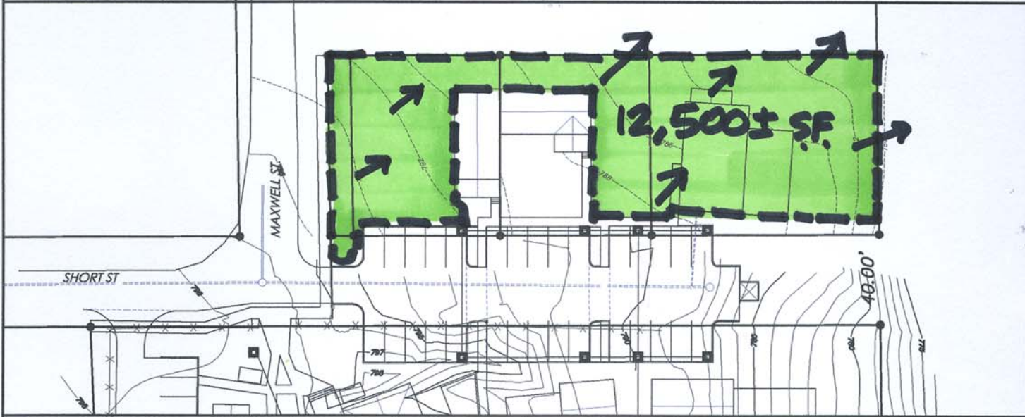
PROPOSED SURFACE DRAINAGE AREA-1
