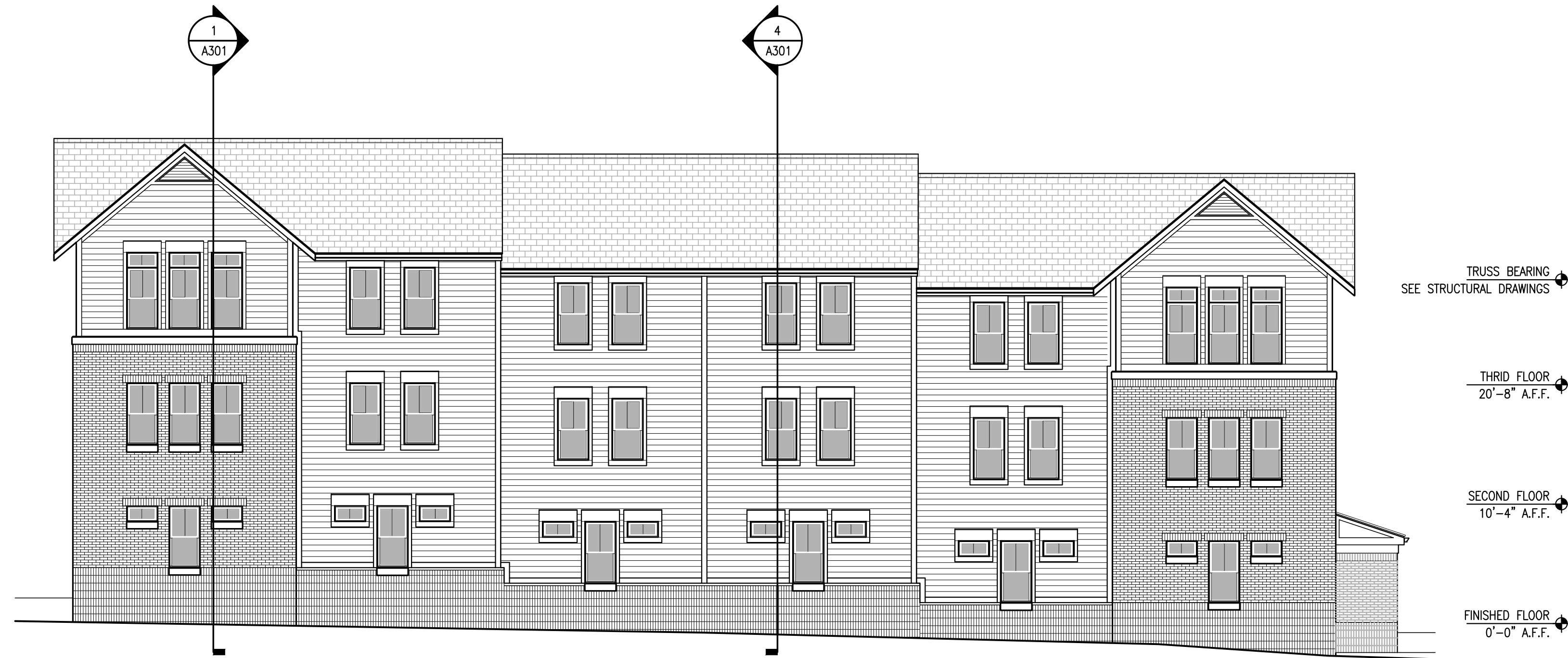
BUILDING 16 SOUTH ELEVATION 3 16A151 SCALE: 1/8" = 1'-0"
