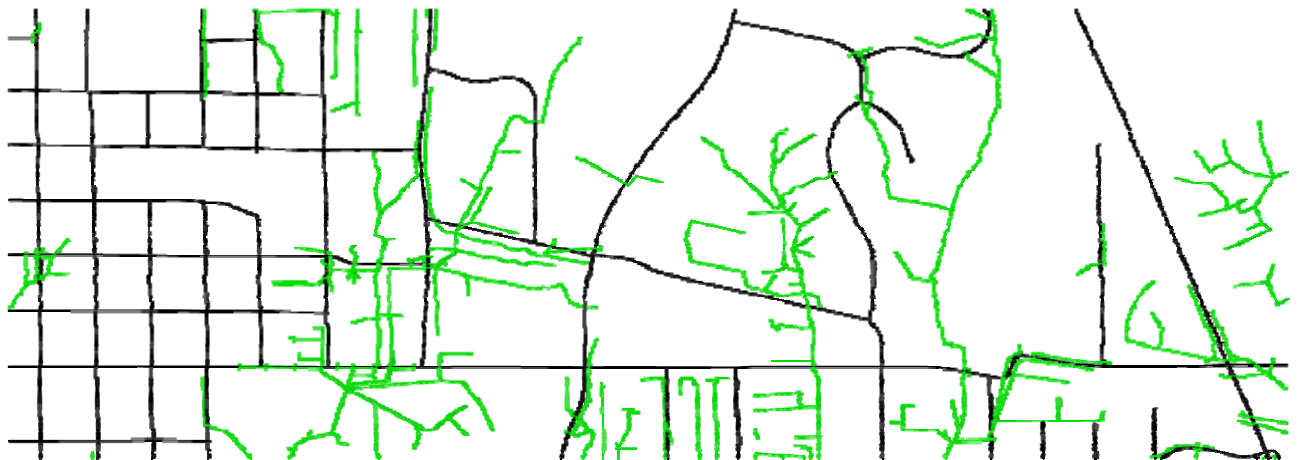
Figure A.5: Map showing locations of existing storm sewer pipelines in green with roads in black (City of Bloomington Utilities 2006).
