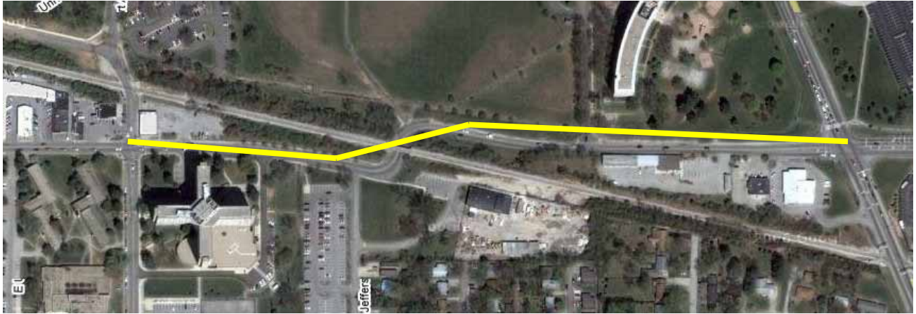
Figure C.20: Proposed realignment of the 10th Street underpass.
