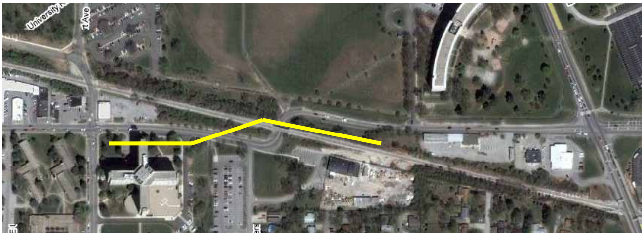
Figure C.21: Proposed at-grade crossing to replace the underpass.
