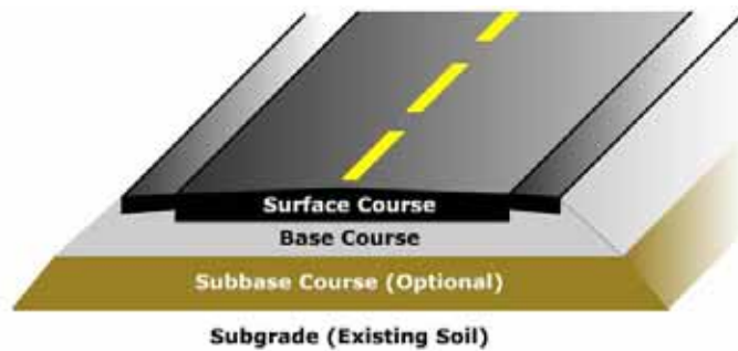
Figure 6: Cross section of pavement design (Washington State Department of Transportation, 2007)
