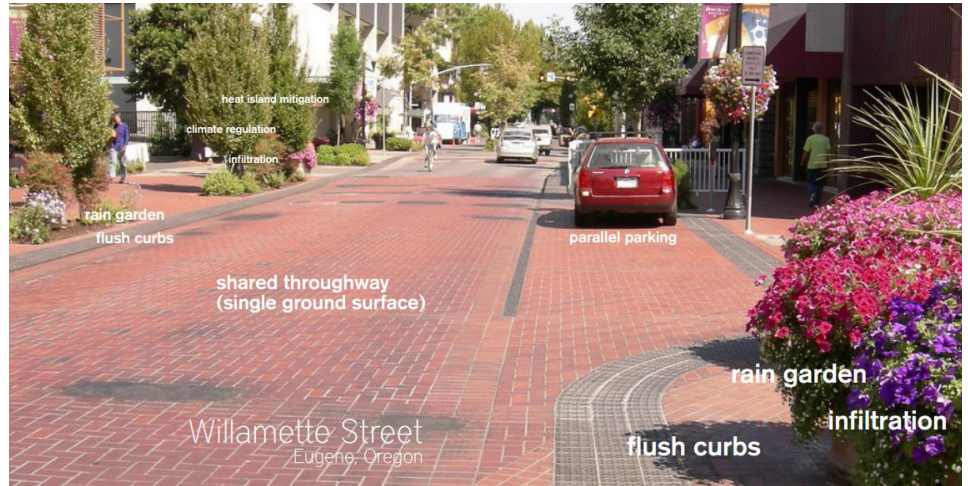
Concept image of a curbless street in Eugene, Oregon. A similar concept will be evaluated for the realignment of 10th Street from Morton to Rogers. Source: LID Manual, bwdh20.org
