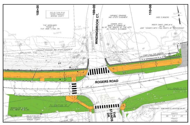
Reduce road width to provide shorter crossing distance (reduced from 44' to 23')
