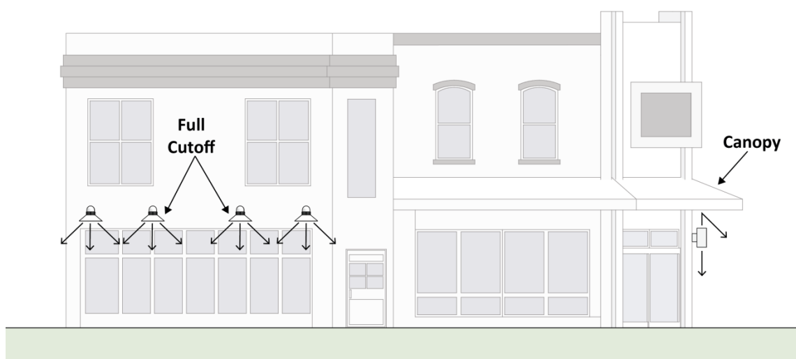
Figure 52: Exterior Light Shielding 928
