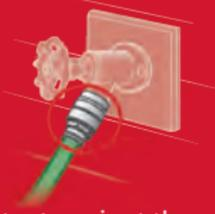
To protect against these common cross-connections, check to see if you have air vacuum breakers installed on each of your hose bibs.
