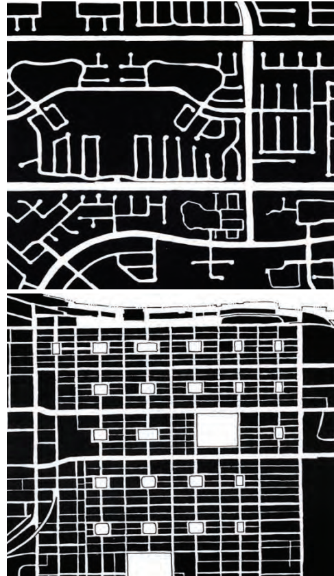
A disconnected street network (top) and a connected street grid network (bottom)
