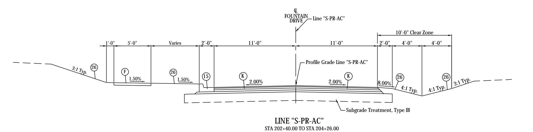
HORIZONTAL SCALE BRIDGE FILE CITY OF BLOOMINGTON 1/4" = 1'-0" N/A RECOMMENDED FOR APPROVAL B-LINE TRAIL EXTENSION & MULTI-USE PATH VERTICAL SCALE DESIGNATION DESIGN ENGINEER 1/4" = 1'-0" 1700735 SURVEY BOOK SHEETS TYPICAL CROSS SECTIONS LINE "S-PR-AC" DESIGNED: BSF DRAWN: BSF 10 of 88 N/A CONTRACT PROJECT CHECKED: LAR CHECKED: LAR R-40193 1700735
