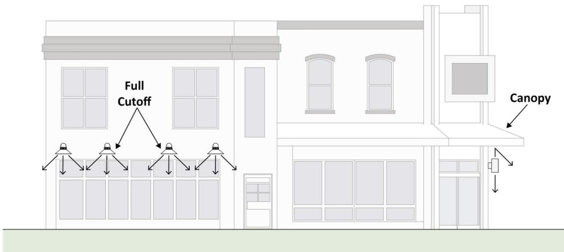
**Figure 51: Exterior Light Shielding**
