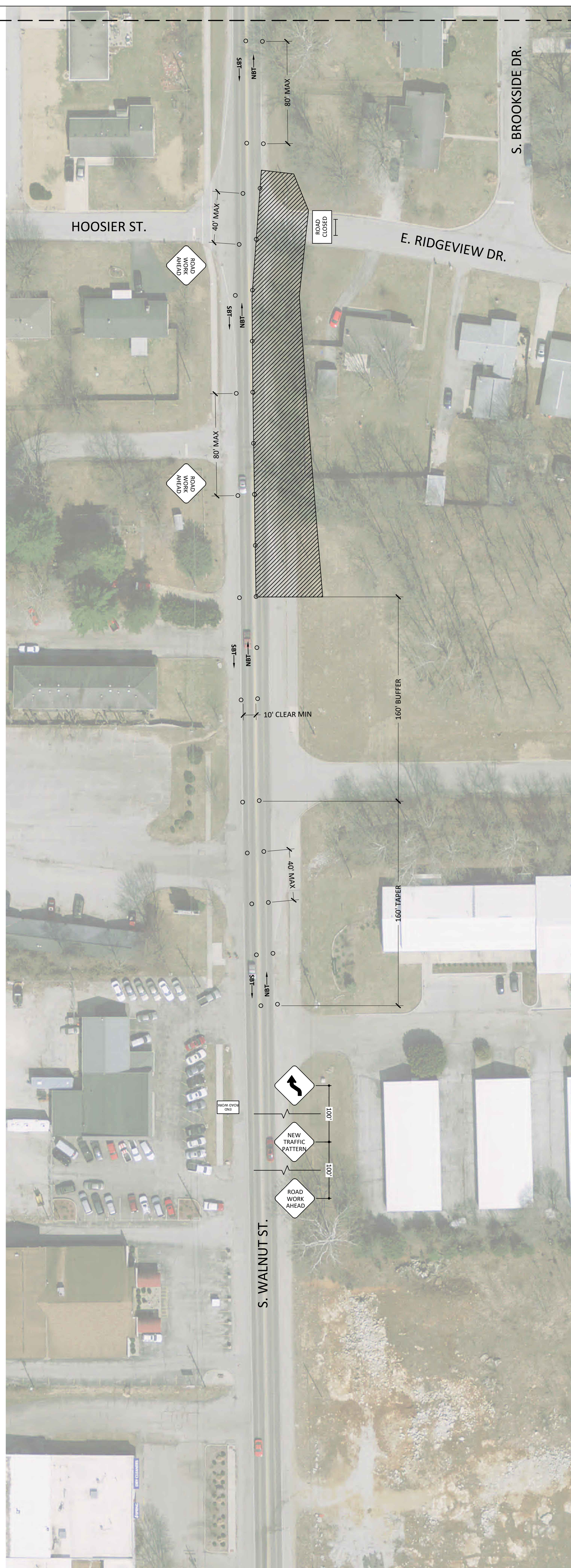
PHASE 1 MAINTENANCE OF TRAFFIC PLAN - SOUTH N.T.S.
