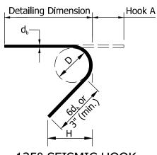
135° SEISMIC HOOK
